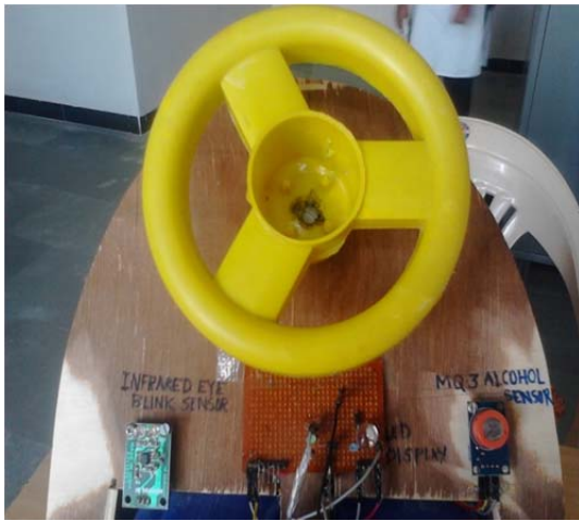
Fig. 5.2: Eye blink sensor and alcohol sensor
